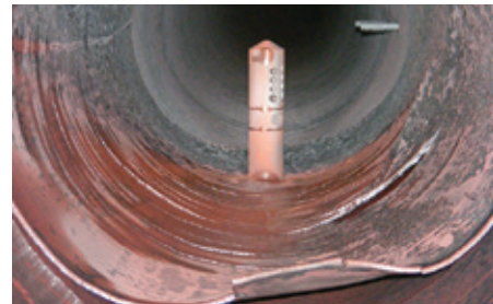
2. Spray-nozzle failures are relatively common in cycling units for some designs of mast-type attemperators (left). Cracking and separation of the liner from the steam pipe downstream of the spray nozzle can occur when relatively cool spray water is allowed to contact the liner (right)
