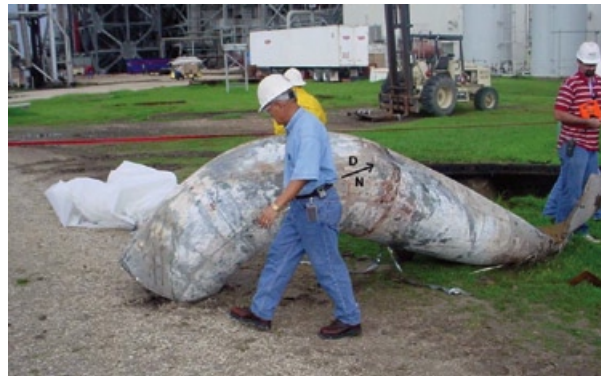
5. Perhaps the most hazardous time in a powerplant’s service life occurs when the plant systems are in an abnormal configuration, with unfamiliar valve and equipment line-ups. This leg of cold reheat pipe became a projectile that, luckily, missed onsite personnel
