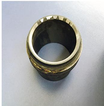
Figure 13: Normal PCV seat wear after 5 years of cycling service.
