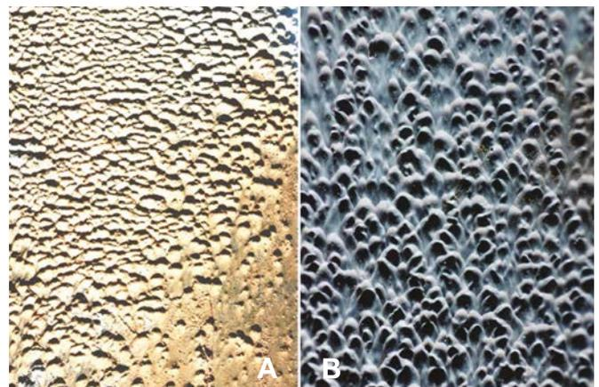
Figure 4: Two views of the visual surface appearance of single-phase FAC. A is a typical detail from an economizer inlet header tube in a conventional fossil plant. Example B is a similar view from the FAC surface near the inlet of an HRSG LP evaporator tube. In both cases the horseshoes or chevrons point in the direction of flow (bottom to top) [4].
